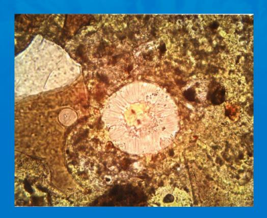
The pore in the middle of the photo is about 110 microns in diameter. The Figure is taken in 40x magnification 320447x70 mm
